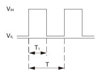
When the PWM control terminal is open, the fan speed is the same as the speed at 0% PWM duty cycle.
