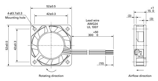
Reference Dimensions of Mounting Holes and Vent Opening (unit: mm)
