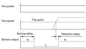
Startup delay: 18±3 s Detection delay: 3 s max. Trip point: 1700 min-1
