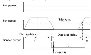
Example 2: when the rotor is locked when the fan motor is turned on and released after the start-up delay time.
